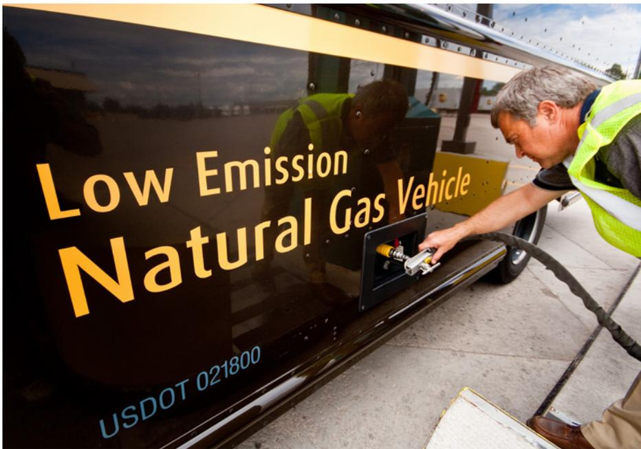
CNG vehicles are fueled with easy-to-use, pressure-sealed fueling connectors. Photo by Pat Corkery, NREL 18188
